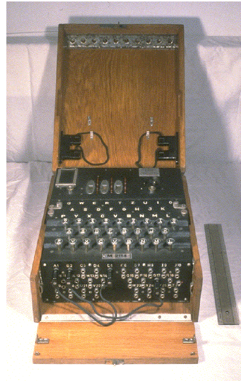
German 3 rotor Enigma Crypto. Machine(1940)
