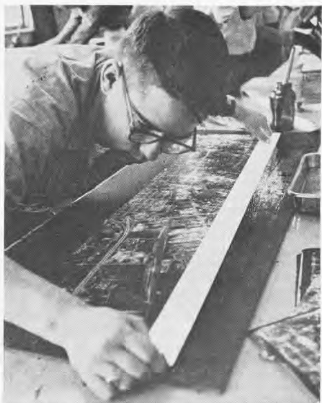
AFTER ADJUSTING image points and cementing photos to the board, PH3 Keller puts on final touch: the border to set off his work.
