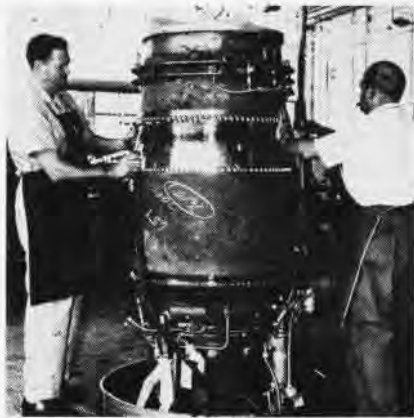
JET TURBINE IS PUT ON HYDRAULIC LIFT
