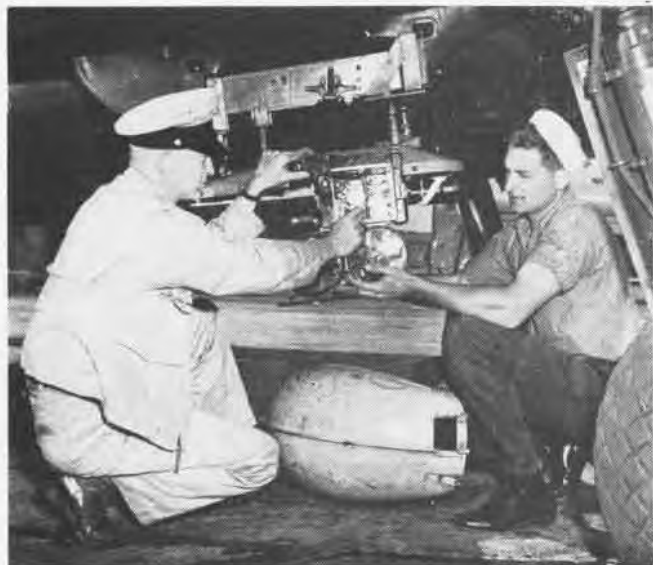
Something new to carrier photo pilots was this movie camera rigged to bomb rack of F6F; drones carried remote control equipment
